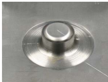
Cylindrical cup formed within Flexform
