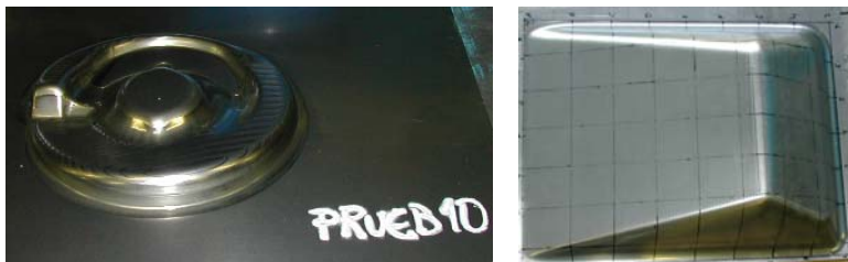
Benchmark parts formed within Flexform to investigate forming parameters
